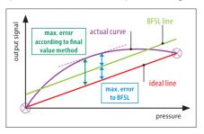
Non-linearity is also shown as BFSL (Best Fit Straight Line) as a reference value in the technical specifications. Non-linearity generally has the biggest influence on the overall error rate. Typically, non-linearity as per BFSL corresponds to half of non-linearity as per the full scale method (1% FS ~ 0.5% BFSL).
