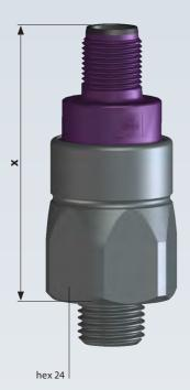
DIN EN 175301-803-A PE 2 1 3 Pin 0601 0602 1 Uv+ Uv+ I<sub>out</sub> 2 Gnd 3  $\mathsf{U}_{\mathsf{out}}$ nc\* IP65  $\mathbf{x} \sim 60 \text{ mm}$  without coupler socket  $\mathbf{x} \sim 77 \text{ mm}$  with coupler socket Order number: 013 AMP Superseal 1.5®
