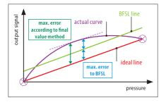
Non-linearity is also shown as BFSL (Best Fit Straight Line) as a reference value in the technical specifications. Non-linearity generally has the biggest influence on the overall error rate. Typically, non-linearity as per BFSL corresponds to half of non-linearity as per the full scale method (1% FS ~ 0.5% BFSL).
