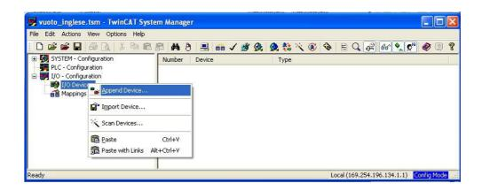
In the Insert Device window select the EtherCAT (Direct Mode) item and confirm pressing the **OK** button.
