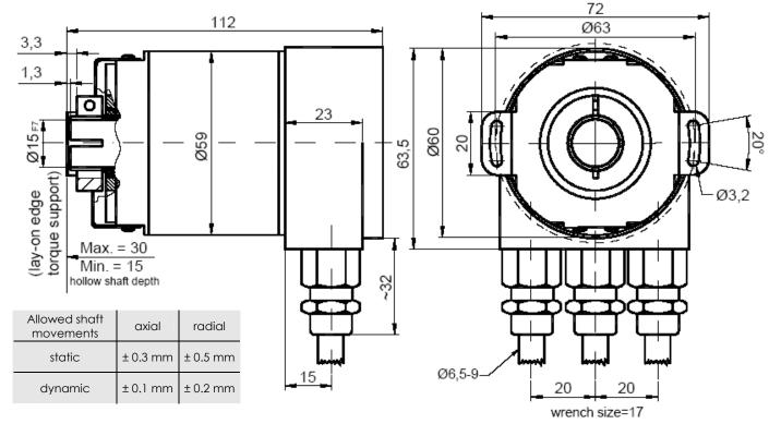
Shaft diameter can be reduced at 12mm, 10mm or 8mm by reduction ring (by slipping them into the hollow shaft)
