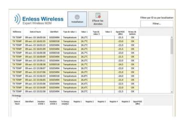
The frames sent by transmitters are displayed in real time according to the transmission periodicity chosen.
