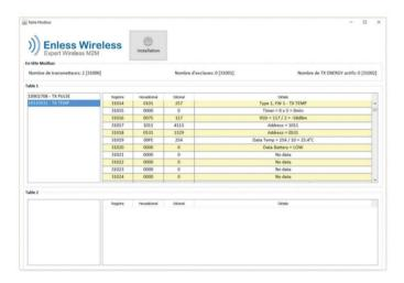
For each transmitter, you will find the addresses of the registers to be addressed as well as the calculation methods to be applied for each register.
