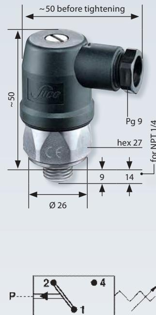
**0141 Piston pressure switches with screw terminals**
