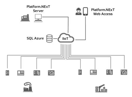
This diagram shows an example of data gathering from various field devices, connected in a single-protocol architecture for IIoT.
