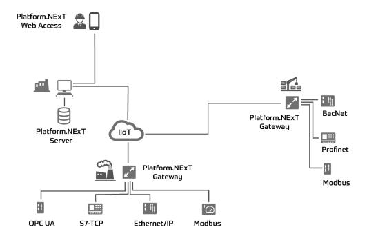
This diagram shows another example of data collection from various field devices, each of which in this case uses a different protocol. In this respect, Platform.NexT's Gateway function is the ideal tool for managing an IIoT project
