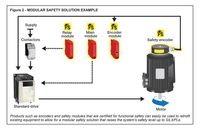
simply swap out older components for new, and in doing so immediately improve a system's overall Functional Safety level. These newer components are often more sophisticated and a single device can sometimes be used to perform tasks that previously may have required multiple devices to achieve the same level of safety.
